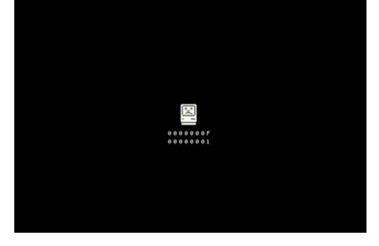
A Sad Mac, just like I saw with MAME in 32-bit mode. I also discovered during this test that on hardware, the same Sad Mac happens in 24-bit mode too. So MAME is actually more tolerant than hardware of that invalid write in 24-bit mode.
