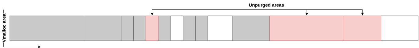
To be effectively freed, the unpurged allocations must be purged. This is done when the number of pages contained in the unpurged allocations crosses the value returned by `lazy_max_pages`, which can easily be computed from userland and is defined as follows:
