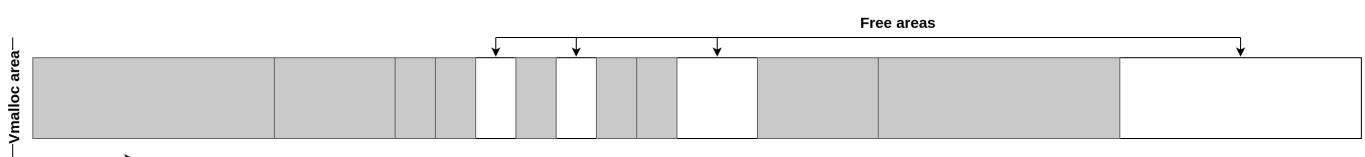
When a new allocation is made, it's placed in the first free area that can accommodate its size. Here is an example for a small allocation that takes the first empty slot:
