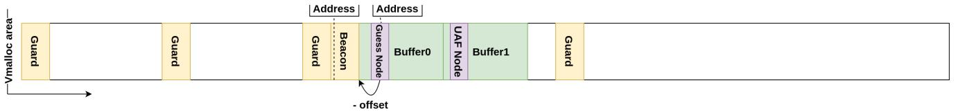
The guess address technique may seem superfluous, but it's essential as we cannot ascertain the exact beacon stack base address from the leak. This ambiguity is due to the `random_kstack_offset` feature and the possibility that a kernel stack allocation can begin at any page boundary.
